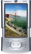
128KB 16MHz Serial 160x160BW 64MB 400MHz Serial/USB/Bluetooth/Infrared 320x480 24bit, Sound, Expansion
